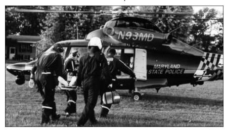
Utilizing the fewest number of personnel necessary to safely load the aircraft within the direct view of the pilot helps to minimize any potential risk.
