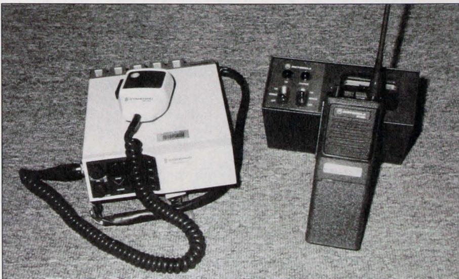
*New radio system: (l-r) Standard GX3000 mobile radio and Motorola MT 1000 with 12 volt battery charger.*
