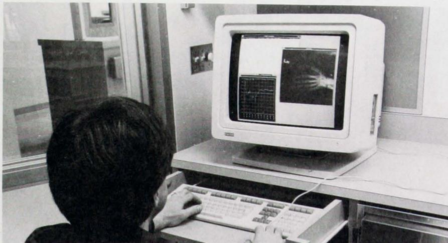
*Bedside workstations have a variety of processing, windowing, and graphics capabilities. These powerful units will store patient data, which will be "dumped" to permanent storage in the computer center at planned intervals.*
