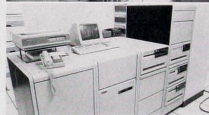
*(Top) PCs to be installed for the secretaries in the new building are lined up in front of two VAX 11/780 units already in operation. (Bottom) In the drawers of this hierarchical storage controller are disk drives containing disks on which information is stored. Disks can be removed and replaced, similar to floppy disks on a PC.*
