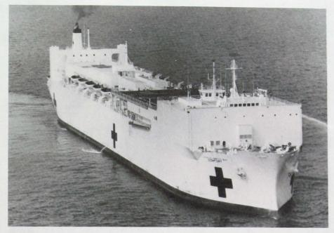
The 894-foot USNS Comfort is equivalent to a 10-story building. The distance from the mast to the water line is 124 feet when the ship is fully loaded. (Photo courtesy of US Navy)
