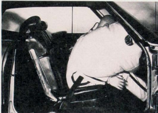
An airbag is located in the dashboard or steering column of a car. In a front-end collision, the airbag inflates instantly to prevent the driver and passengers from hitting the windshield or dashboard. It inflates and deflates so rapidly that people involved in accidents are hardly aware it has operated. (Photo courtesy of U.S. Department of Transportation)
