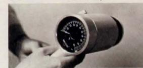
A radiometer is used with biofeedback techniques to indicate the patient's hand temperature.
