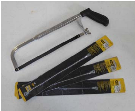
Hacksaw, with three (3) carbide wire type blades
