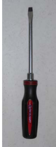
Screwdriver, 12", standard slot blade
